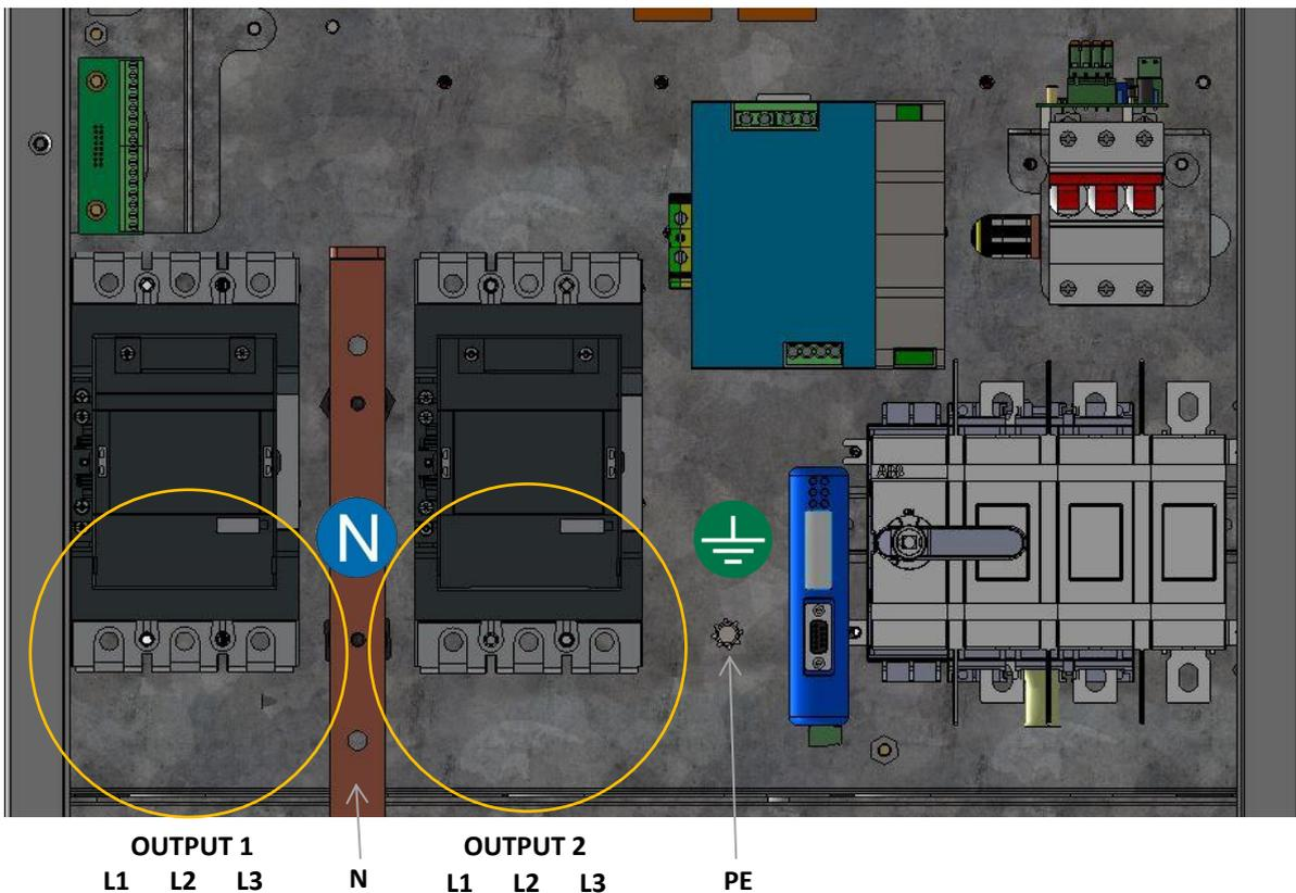
Additional ferrite rings are supplied loose with the PV90-4 GPU, these are for each 400Hz Output and should be fitted to the output cable/s at the time of installation. These rings help reduce output electrical noise to the aircraft. Note: Ensure all 4 cores (L1, L2, L3 & N) pass through the rings in the same direction.
