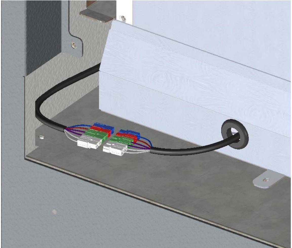
3. Disconnect the Fan Assembly Plug/Socket Connector, as shown above.
