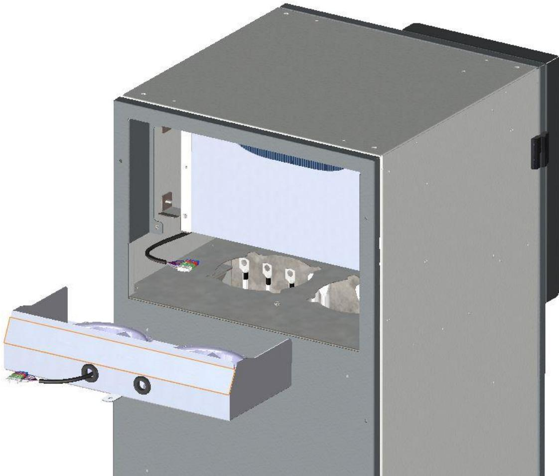
4. Remove the Fan Assembly by sliding it out.
