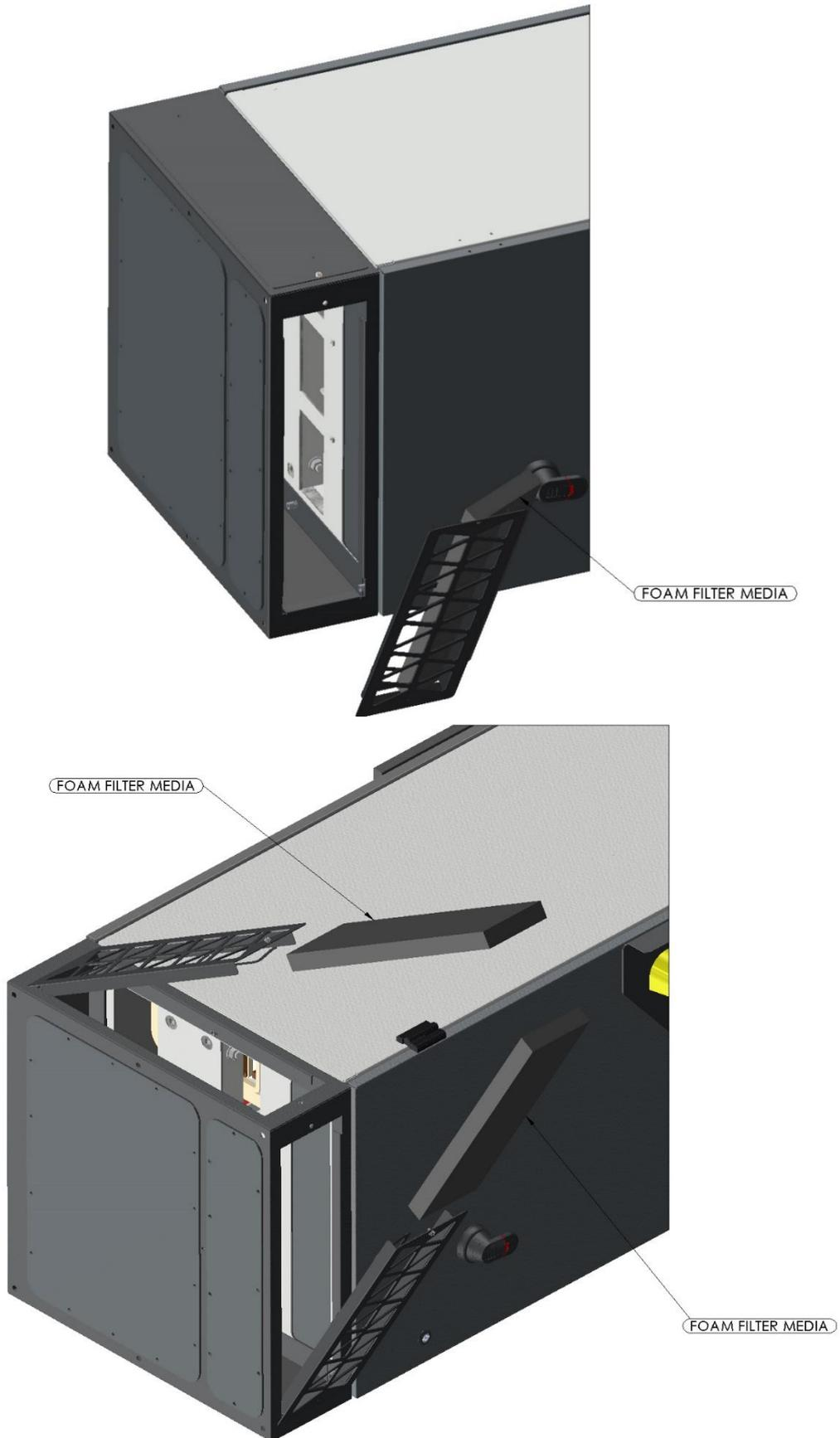
3. Restore the filter media metalwork and ensure the fixings are secure prior to re-energisation.
