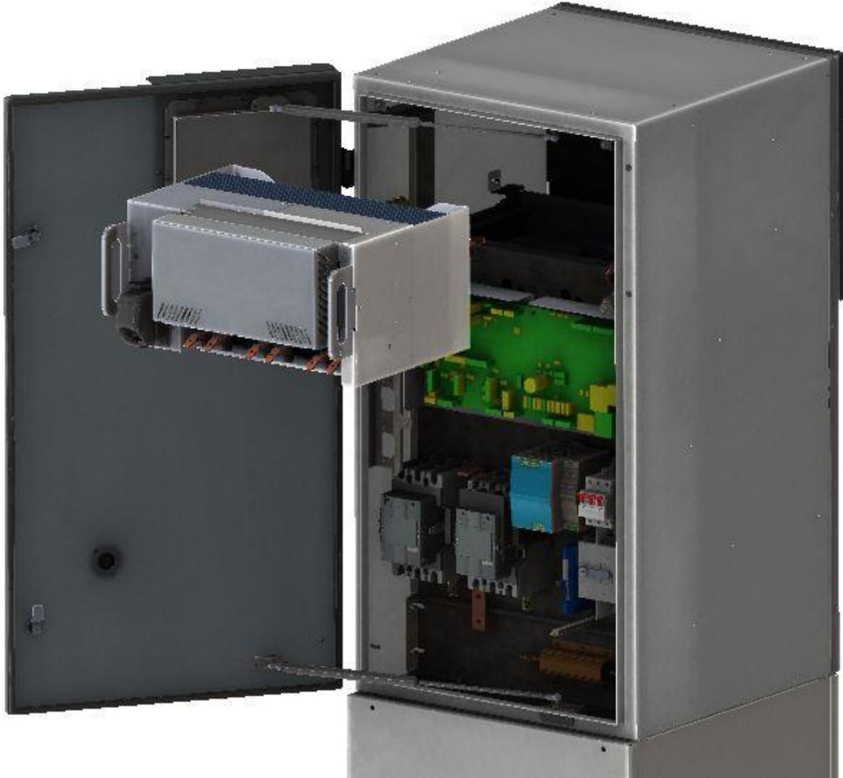
8. The power module can now be replaced. Ensure the Power Module is secured into position and the retaining brackets are re installed
