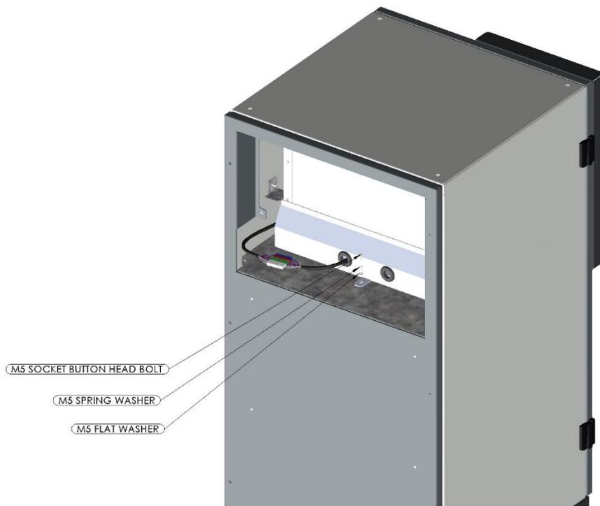
2. Remove the Fan Tray Fixing Bolt as shown above.
