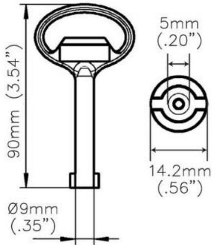
Both front and rear doors use the same key, the image to the left provides details of this key for future reference.
