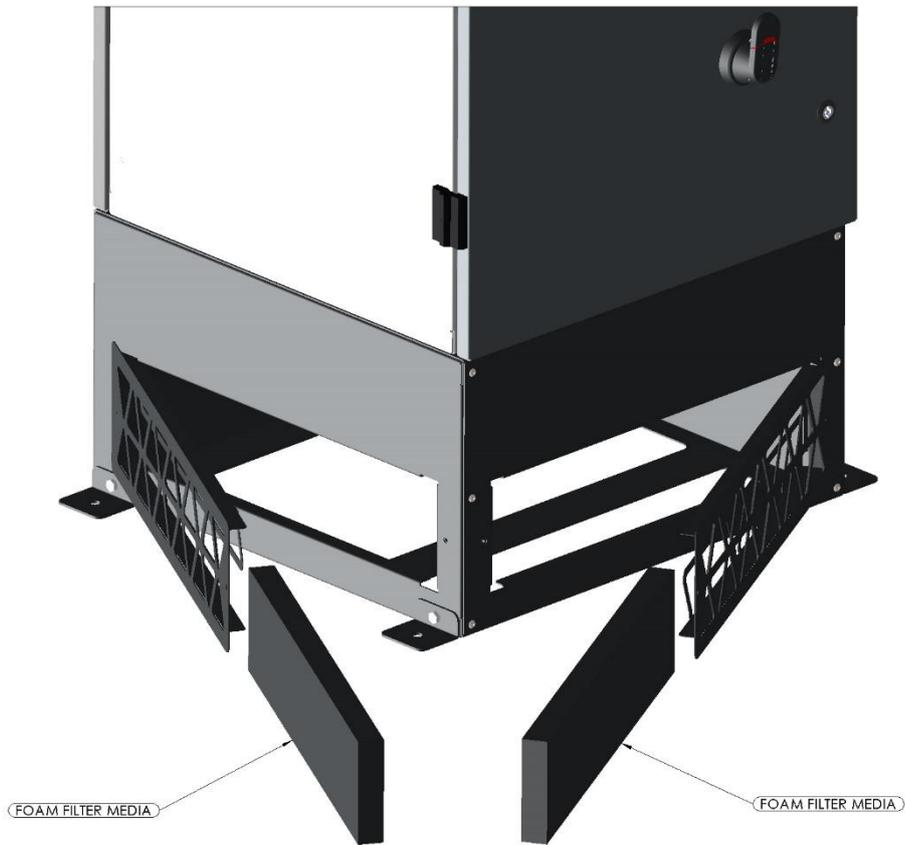
4. Replace filter cover panels. Restore the filter media metalwork and ensure the fixings are secure prior to re-energisation.
