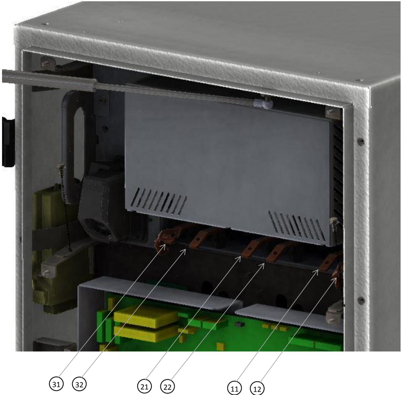
6. Connectors marked PL1 and PL2 must be then disconnected from the power module. PL1 is removed by pulling on the lever; PL2 is loosened via the screws either side of the connector.
