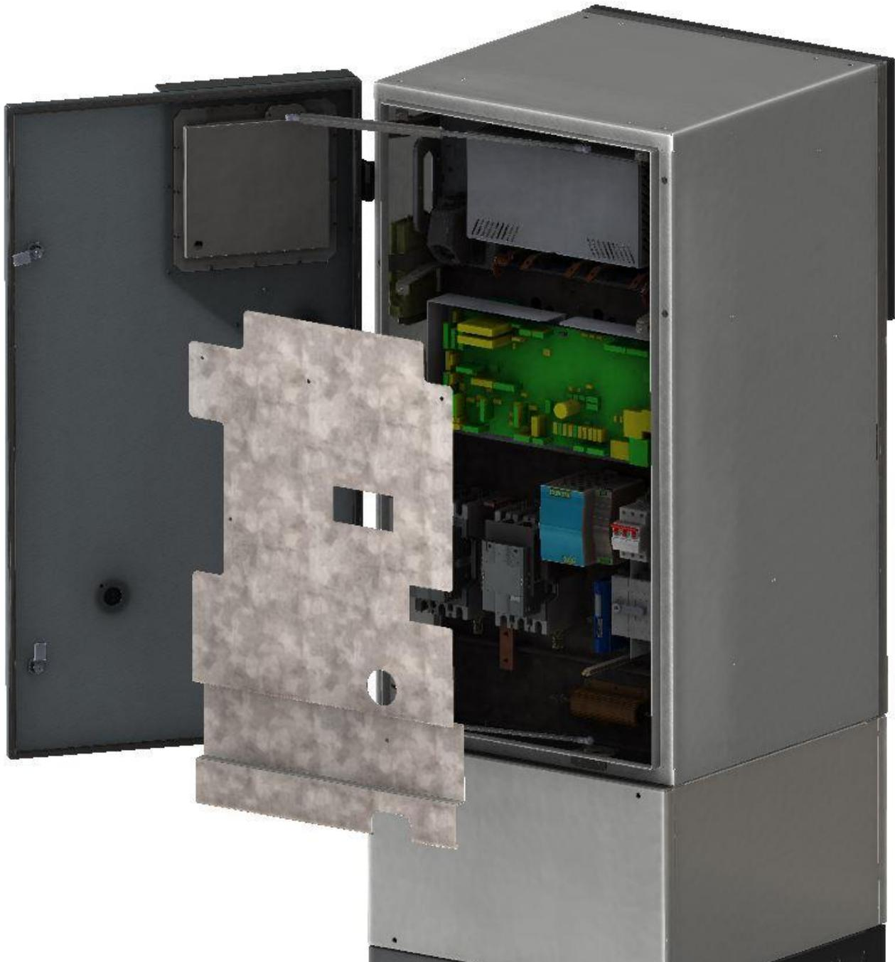
5. Measure between cables 11,12,21,22,31 & 32 with a voltage meter to ensure there is no voltage remaining on the DC capacitors (measure between each connection and earth). Then disconnect the 6 x cables as illustrated below.
