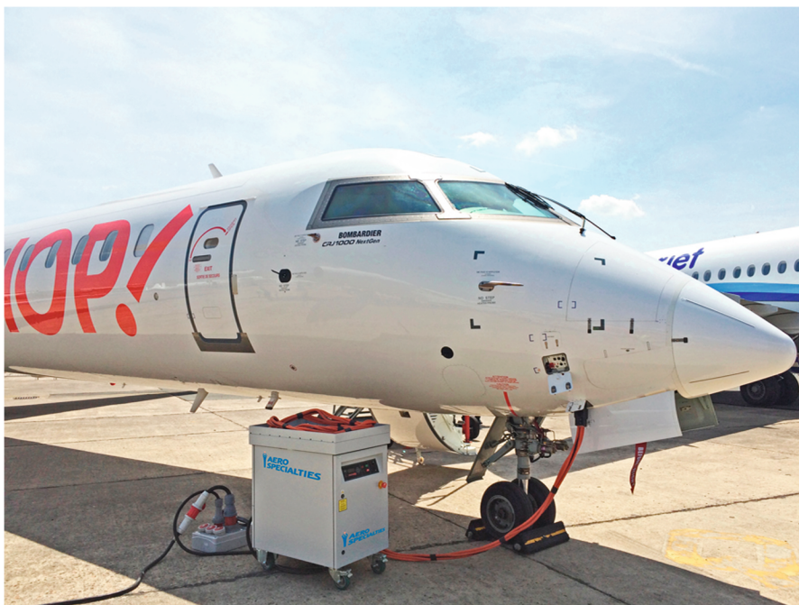
PV45: powering Bombardier CRJ1000
